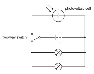
complete circuit and two lamp symbols; correct parallel arrangement;
